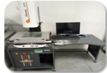
Optical meter Function: Length, curvature, area. Accuracy: \pm 5\mu\text{m}
