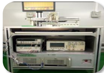
Automated crystal oscillator test machine Function: Crystal resonator test
