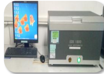
XRF Spectrometer Function: ROHS material test
