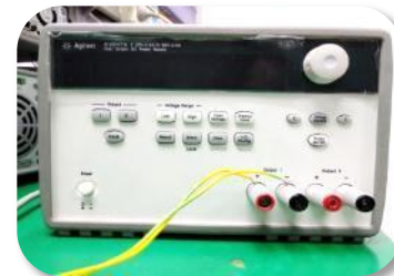
Stabilized voltage supplier Function : Provide DC voltage
