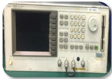
Network analyzer Function: Frequency and resistance test
