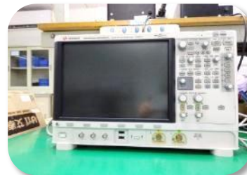
Digital oscilloscope Function : Waveform test
