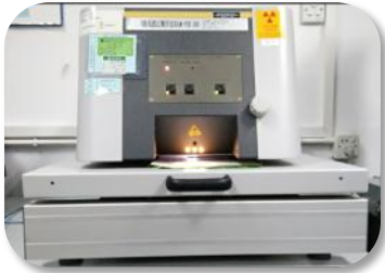
X-ray film thickness tester Function: Film thickness test
