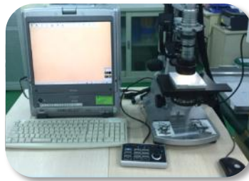
3D electronics microscope Function: Magnification rate :1200 times, Accuracy: 0.005mm
